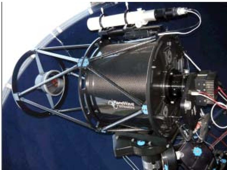
*Planewave 0.5m astrograph fitted with a FLI Proline PL1002M CCD camera. This package is stationed in New Mexico.*
